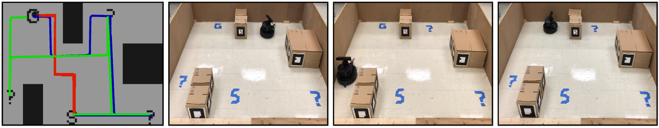
Fig. 2. Demonstration of the path taken by the robot with three different initial beliefs for the map in Figure 1. The start state and the true goal state are denoted by S and G, respectively. The other potential goals are denoted by the question mark symbol. Green, blue, and red show the path taken by the robot with 0.1, 0.25, and 0.9 as the initial belief for the true goal state and equal probability for other potential goal states.
